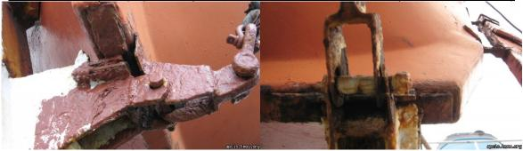
Picture of other deficiency: STOWAGE OF LIFERAFT (P.S.) - WEAK LINK IS
